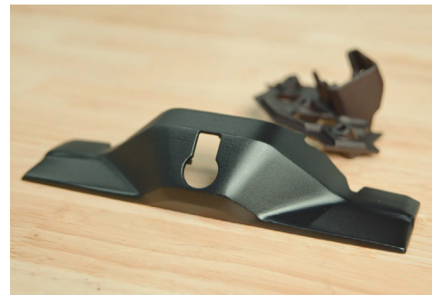
The 3D printed camera mount bracket with retention clip shown behind.
